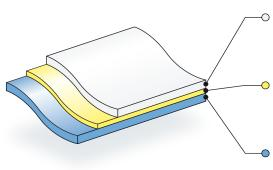
**Facestock:** 2 mil optically clear scratch resistant topcoated polyester that offers excellent clarity and dimensional stability combined with good high temperature and humidity resistance. The optically clear polyester provides high resolution imaging with excellent adhesion to UV curable inks.
